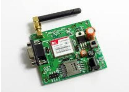
Fig 1: GSM module
