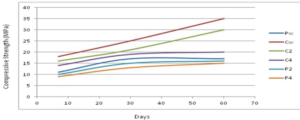
Figure-1: Compressive strength of Samples under various curing options
