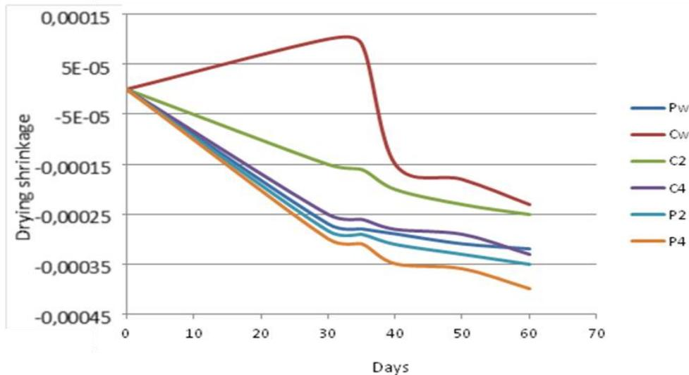
Figure-3: Shrinkage result of evaluated samples under various curing options
