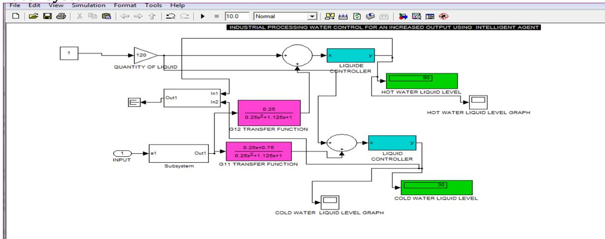
**Figure: 5** System without Intelligent agent for increased output
