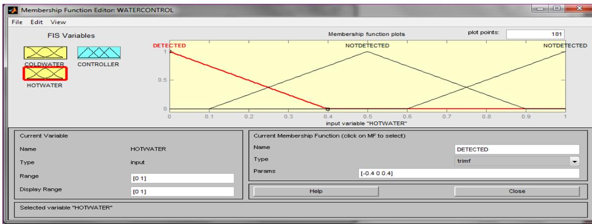
**Figure: 3** Design of a membership function that will detect irregularities.
