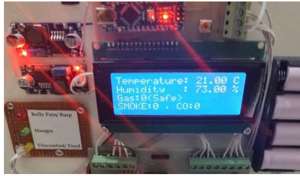
Figure 9: Ensuring safety by monitoring different environment parameters (LPG, CO gas, smoke, humidity and temperature)
