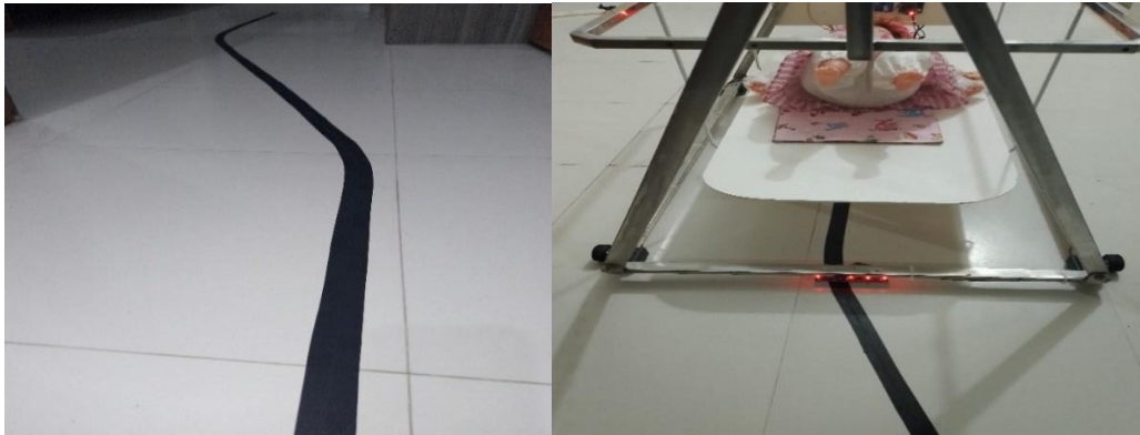
Figure 12: (a) Path for traverse of Baby Nursing Robot (b) Line detection of the cradle.
