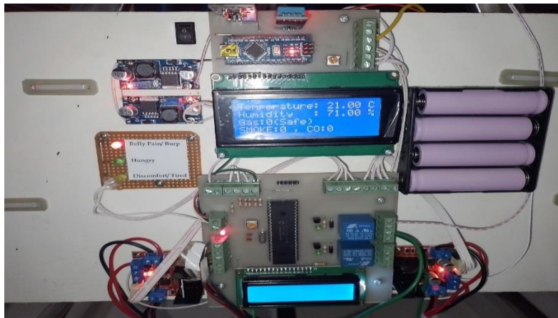
Figure 10: Detection of Belly Pain/ Burp cry after sound play through LED
